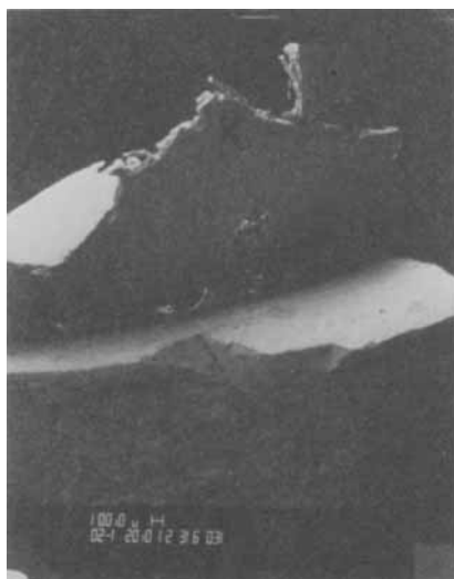
FIGURE 12 SEM picture of debond region of a medium wedge test joint (STAB(1)).
