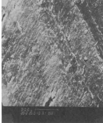
FIGURE 18 SEM picture for debond region (adhesive, position 59 Figure 16) in a bad wedge test joint (STAB(1)).
